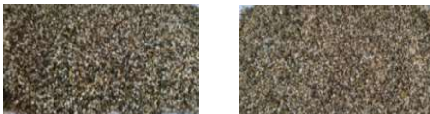
Figure 3 Different size gravel (average 5 mm and 2 mm in diameter) used in slow sand filtration system
